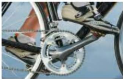
Your foot exerts a torque that rotates the crank.
